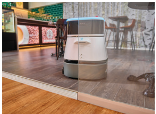
The co-botic™ 45 can recognize transparency and move around see-through obstacles when needed.
